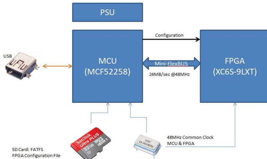
To support the potential uses of the hardware a firmware stack is also provided, that enables programming the FPGA configuration from the SD card, and provides the access methods to the FPGA side along with drivers for Serial, USB, SD, FATFS etc. The stack is based on a modified version of FunkOS RTOS, and the extensions provided are developed using TDD to ensure high quality and reliability of the system.
